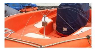
On Saracen, the white wooden bracket for the spider mount fits onto the track fixed to the front of the console (once again, after the cover has been fitted)
