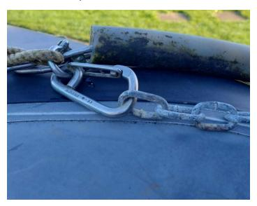
To moor the boat, release the carbine hook from its storage place on the eye in the floor of the boat. The chain is encased in a clear plastic pipe and is permanently attached to the Dring on the outside of the boat under the bow. Then lift the mooring buoy onto the side of the boat and attach the carbine hook to the chain below the buoy. Lower the mooring buoy back into the water.
