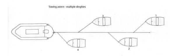
In a "herringbone" tow as illustrated above, each dinghy helm will need to put about half centreboard down, and then steer the boat using their rudder to maintain the position of the dinghies as illustrated.
