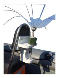
On Jaffa 1, the shorter spider, which has a larger mounting pole (25mm diameter) is mounted in the finger hole of the anchor-well lid.
