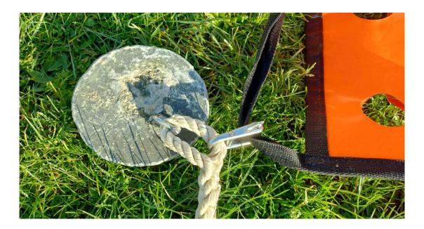
Note the captive shackle used to attach the racing mark to the warp.
